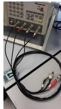
Figure 9: LCR meter test clip with 4 BNC cable
