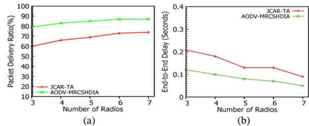
Figure 4: Results of varying the number of radios
